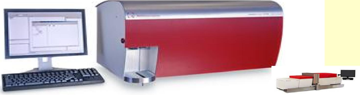
Fatty acid calibration was done once per month with reference milks produced at Cornell. The instrument tests about 50 to 70 samples per hour for all components, NPN/urea, and all fatty acid parameters. The automated model runs 600 samples per hour.
